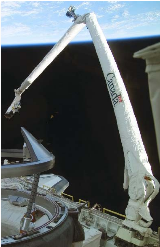
Canadarm is a robot arm on a spaceship Photo: Courtesy of NASA
